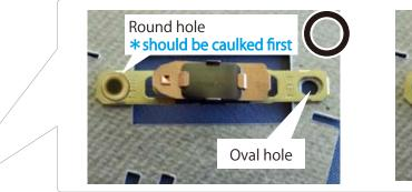
**STEP 1:** At first, put Eyelet through Round hole and caulk it.
