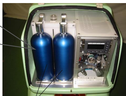
Cartridges filled with Fe/Fe 3 O 4 pellets
